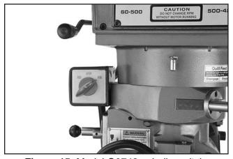
Figure 15. Model G0748 spindle switch.
